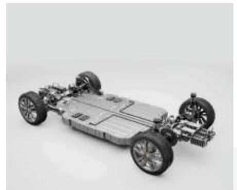
BATTERY AS PART OF THE CHASSIS
